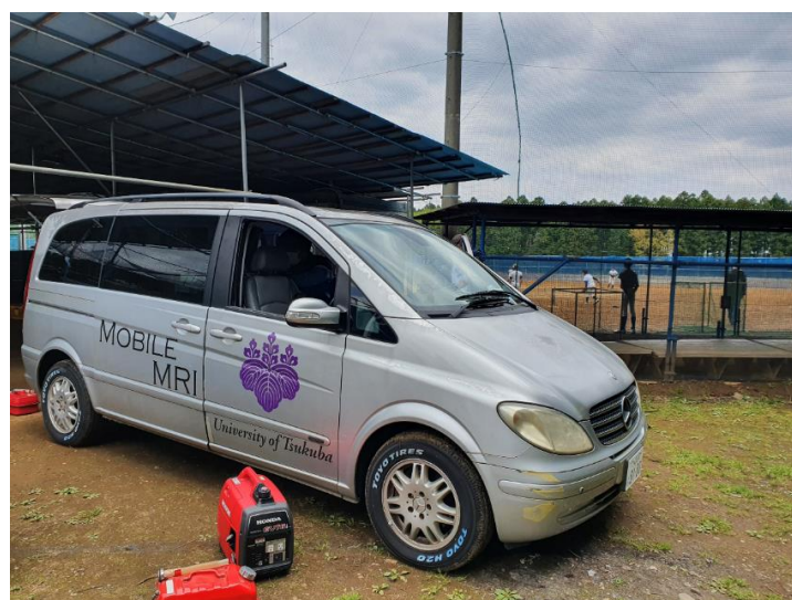
Figure 1. Photograph of the mobile magnetic resonance imaging (MRI) system beside a baseball field. (Mercedes Benz, GH-639811, width 191 cm, height 193 cm, and length 476 cm). Mobile MRI enables players to practice while awaiting their turn for an MRI scan.
